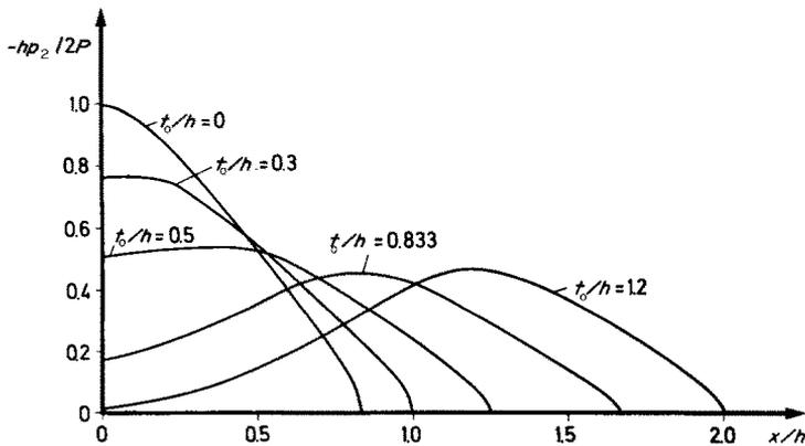
FIG. 5. The distribution of contact stress for various values of  $t_0/h$ , ( $\beta = 1.0$ ).
