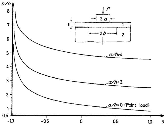
FIG. 6. The variation of contact width with  $\beta$  for loading by a flat stamp.
