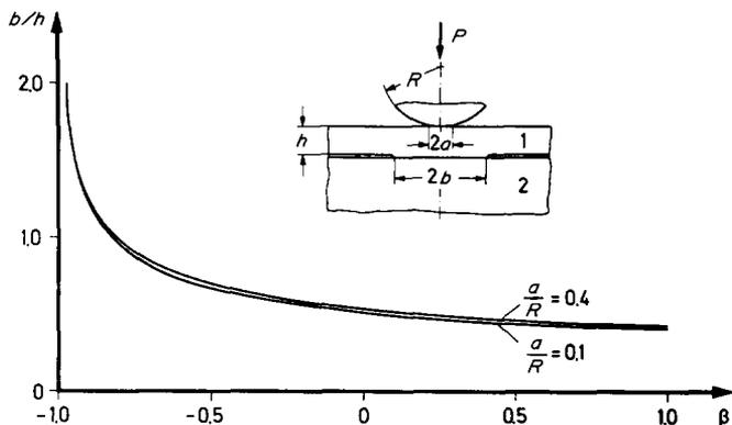
FIG. 8. The variation of the layer-subspace contact width with  $\beta$  for loading by a curved stamp, ( $R = h$ ).
