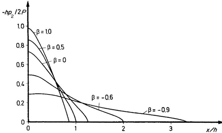
FIG. 4. The distribution of contact stress for various values of  $\beta$ , ( $t_0 = 0$ ).
