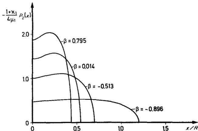
FIG. 10. The distribution of the contact stress between the layer and the subspace, ( $a/R = 0.1, h = R$ ).
