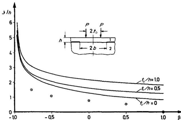
FIG. 3. The variation of the contact width with  $\beta$ . The circles correspond to the result given in [22].
