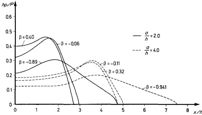
FIG. 7. The pressure distribution between the layer and the half space for various values of  $\beta$  and for loading by a flat stamp.
