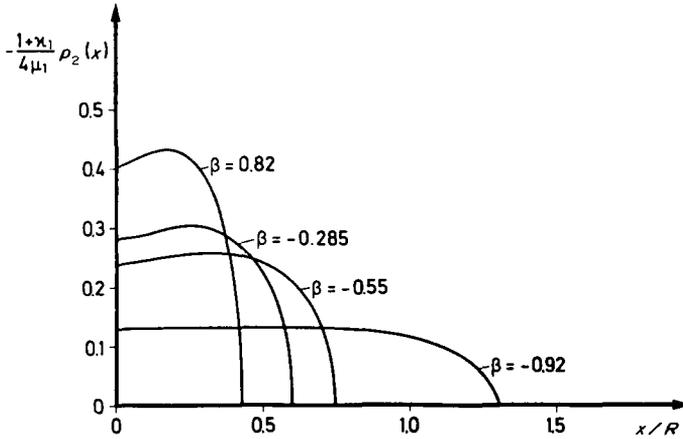
FIG. 11. The distribution of the contact stress between the layer and the subspace, ( $a/R = 0.4, h = R$ ).
